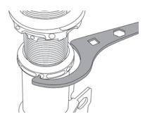
It is important to insert the end of the spanner into the locating hole of the lock rings for a sure grip.
