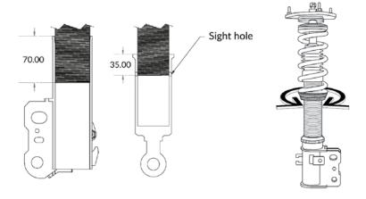
Shock body is threaded into lower bracket until thread is visible. If there is no sight hole, see the specifications in the warning section above.
