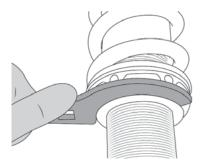
Rotate the lock rings with the included spanner to raise, lower, tighten, or loosen.
