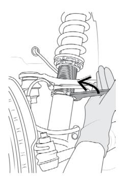
Be sure to tighten the lower lock ring before taking the vehicle for a test drive. It is crucial that the lock ring is secured either by torquing it to the specification listed in Section 7 of the previous page using a torque wrench, or by firmly tapping the spanner with a mallet until the lock ring is fully tightened.
