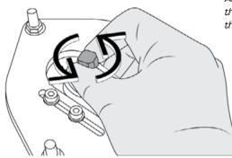
Adjust the shock dampening with the adjuster knob. Do not force the adjuster past the limit stops.
