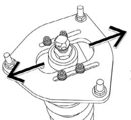
Camber is adjusted by sliding strut laterally relative to camber plate.
