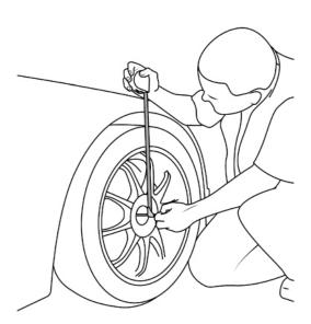
Use a tape measurer and a straight object to measure the wheel gap.
