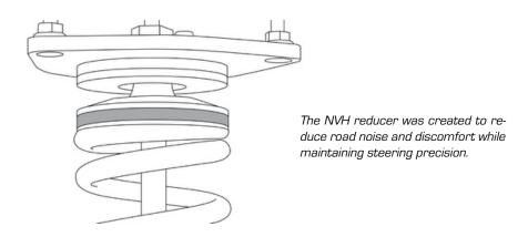
On applications using a front strut design, high-quality Koyo® sealed bearings are incorporated into the suspension top hat/camber plates to increase steering feedback. These bearings also reduce steering effort and suspension noise, as they allow the spring to rotate freely during steering rotation.
