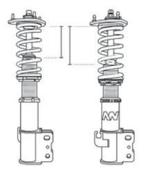
FASTROAD PRO™ was designed to have more usable stroke than typical coilovers resulting in superior grip and comfort.
